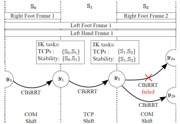
Fig. 6: Robust generation of a feasible path using a contact sequence  $[\mathbb{S}_0, \mathbb{S}_1, \mathbb{S}_2]$ .
