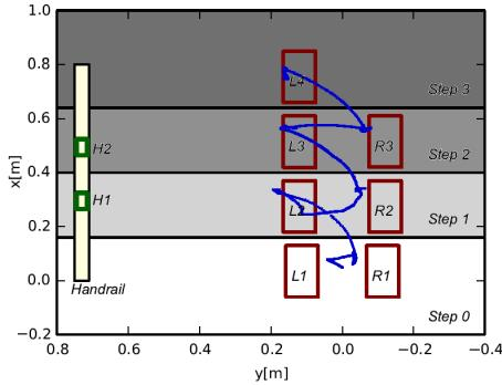
Fig. 8: Planned CoM Trajectory for the stair setup. The contact sequence is  $[L_1, R_1]$ ,  $[L_1, R_1, H_1]$ ,  $[R_1, H_1]$ ,  $[L_2, R_1, H_1]$ ,  $[L_2, H_1]$ ,  $[L_2, R_2, H_1]$ ,  $[L_2, R_2]$ ,  $[L_2, R_2, H_2]$ ...
