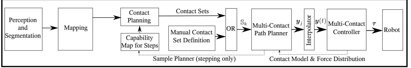
Fig. 1: Pipeline used to generate quasi-static motions either from perception input (for stepping only) or manual annotations (using additional hand contacts).
