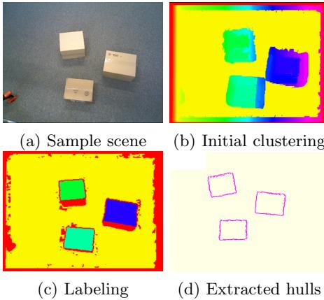
Fig. 2: Segmentation process on depth and normals: a) Color image of a test scene; b) Output of flood fill clustering; c) Clusters of interest with different labels after they were grown; d) Hulls delimiting the flat surfaces.
