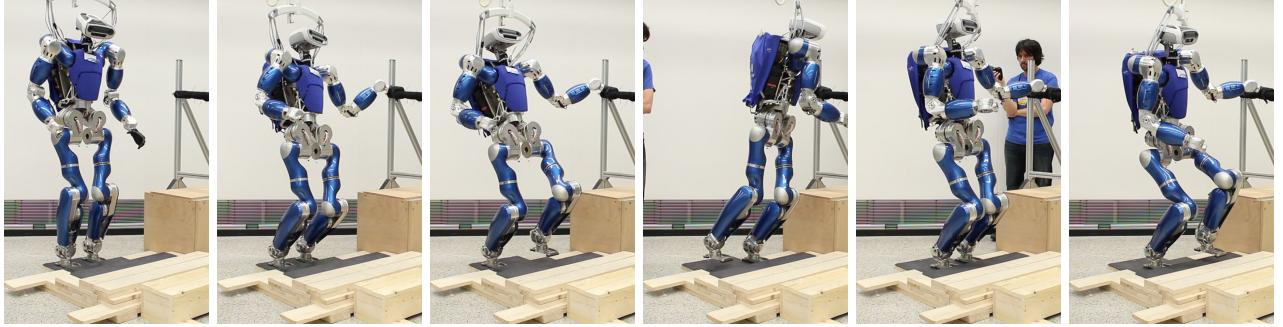
Fig. 7: Snapshots of the experiment climbing stairs. The main challenge of the experiment lies in the correct use of the handrail to support the robot weight, the height of the stairs is 0.05m. The poses were optimized to have the CoM as close as possible to the supporting foot, which results in quite large motions in the joint space.
