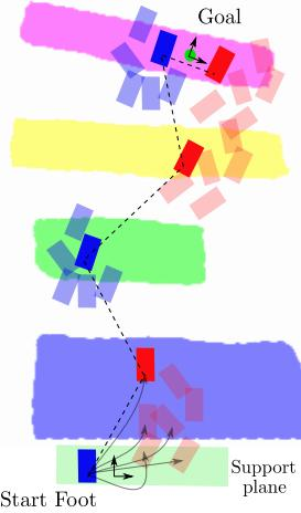
Fig. 4: Generation of a feasible path on the set of hulls.
