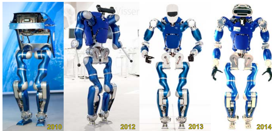
Fig. 1: The torque-controlled humanoid robot TORO and its development stages from 2010 (DLR Biped [1]) to 2014.
